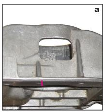
For positioning the new bushing, draw a line like the one on the picture.
