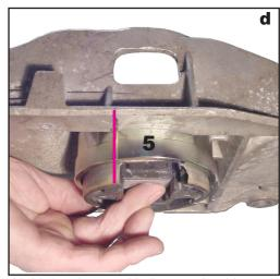
Hold the sleeve with the new bushing underneath the eye of the engine mount. The side of the gap, the mark on the sleeve and the drawn line on the engine mount have to be in line, then ....
