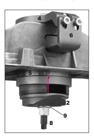
.... assemble the tension bolt, the thrust pads the same way as on the picture. Press in as far as possible.
