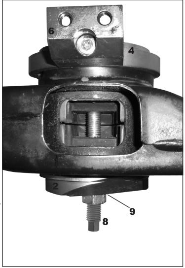
Pull in the bushing. Watch through the "window" for the proper installation height. **Caution!** The pressure sleeve (5) will fall down as soon as the bushing is through.
