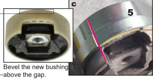
Lubricate the new bushing and the eye in the engine mount. Then push the new bushing into the pressure sleeve (5). The mark on the sleeve must be in line with the gap of the bushing.
