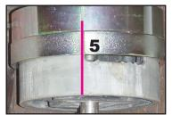
Lubricate the new bushing and the eye in the engine mount. Then push the new bushing into the pressure sleeve (5). The mark on the sleeve must be in line with the gap of the bushing.
