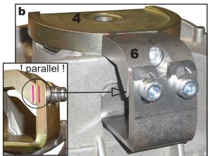
Put thrust pad (4) with the routed side upwards on top of the eye. Screw in the sliding piece (6) and close the "window". Fill the "window" up to the upper edge. You can easily adjust the position because of the longholes.
