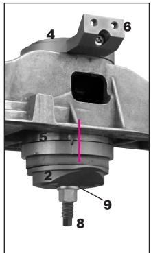
Unscrew the sliding piece (6). Turn over the thrustpad (4). Then assemble the tension bolt, the thrust pads the same way as on the picture.
